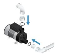
Tighten the pump fittings at the suction and discharge hand tight only. The pump fitting utilizes an o-ring seal that is all that is required for a leak free joint.
