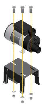
After completing the Pre-Installation Checklist, position the Pump and applicable Pump Stand.
